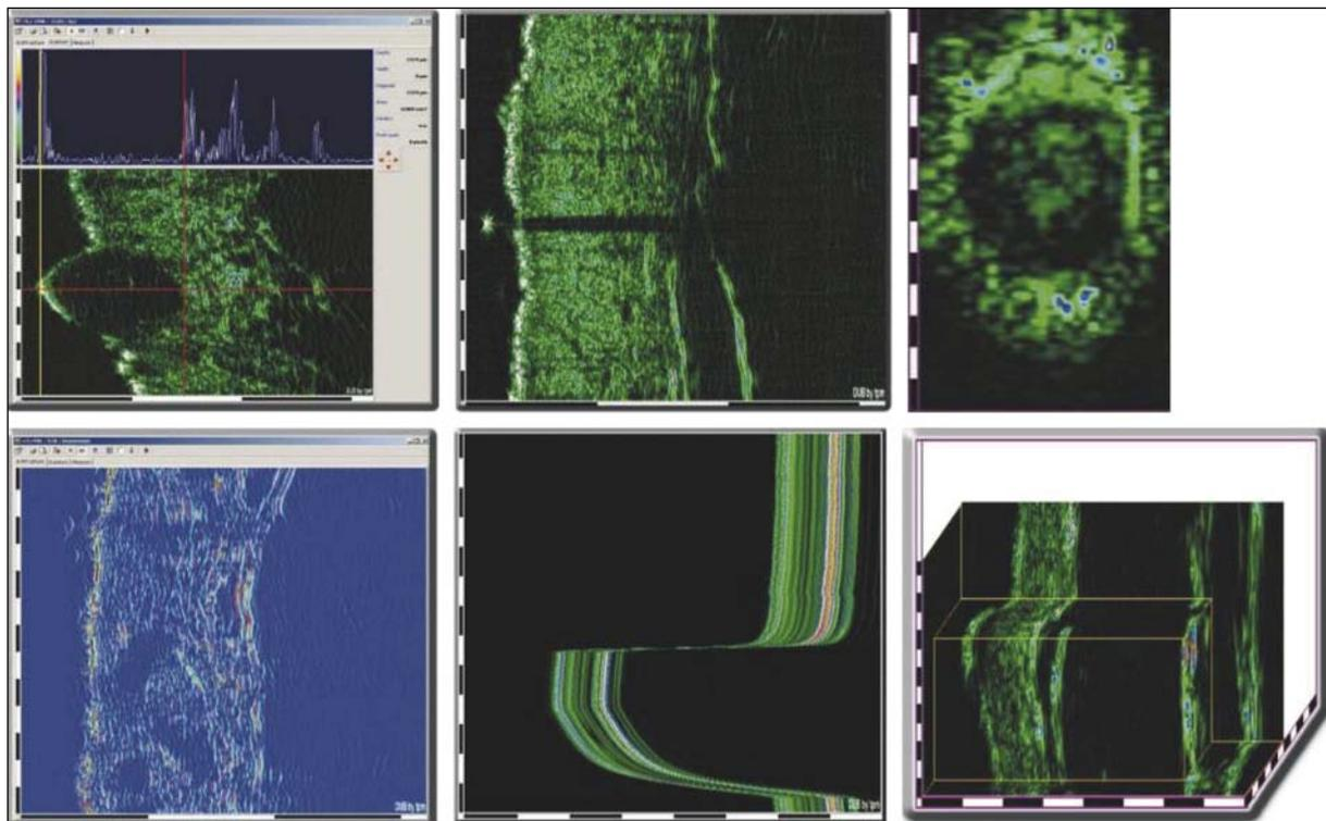
**Figure 4.** Different types of ultrasonographic signal processing. Top (left to right): A-Scan, B-Scan (built up from 384 high frequency A-Scans), C-Mode (3D scan in horizontal cuts in different vertical layers [depth]), Bottom (left to right): RF-Scan (Raw data behind the recorded image), M-Scan (Skin elasticity measurement with high frequency digital ultrasound with a Vacuum Elasto Pump), 3D-Scan (From 10-30 parallel B-Scans). (Used with permission of Taberna Pro Medicum, Lüneburg, Germany).
